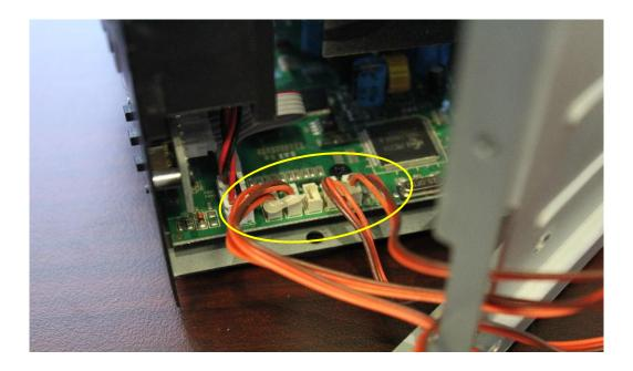
10. Remove the LED(s) from the front panel by removing the screw. Install the new LED(s) using the same process.
