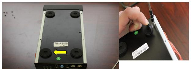
\*Do not completely pull off the foot. Only peel it back far enough to expose the screw.
