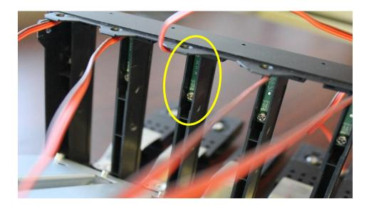
11. Plug in the LED(s) connector back into the PCB in the same order they were taken out making sure the cable(s) goes through the hole in the metal side panel.
