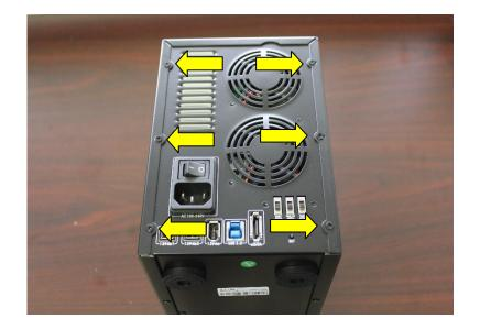
2. Turn unit over and remove the 4 screws on the bottom of the unit.
