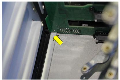
**NOTE:** When putting back on the metal side panel make sure the PCB is place back into the plastic notch on metal side panel.
