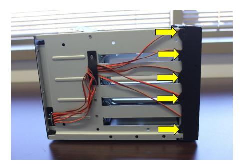
7. With the front panel screws removed, remove the 5 screws holding on the metal side panel.
