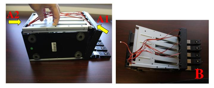
9. Locate the LED(s) that are faulty and trace the cable back to the PCB where it is connected. Remove the glue around the connector(s) and unplug the connector of the faulty LED(s). In this example, the LED for bay 3 is removed.
