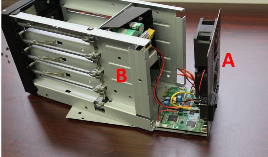
5. Disconnect all wires from the power supply, leaving them only attached to the unit.
