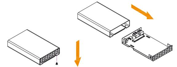
b) Install the hard drive and mount it with the included 4 silver mounting screws. Do not over-tighten.
