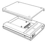
b) Connect the hard drive to both connectors. Place the hard drive into the chassis. The screw holes should align with the mounts.
