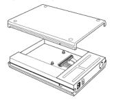
b) Connect the hard drive to both connectors. Place the hard drive into the chassis. The screw hole should align with the mount.
